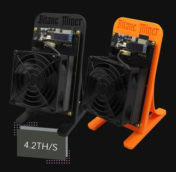
Bitaxe Hex is a **fully open-source Bitcoin** ASIC miner equipped with 6 BM1368 ASIC chip from Antminer's S21.
